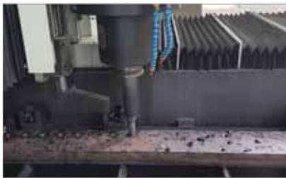
**Cutting condition**  $vc(\text{m/min})=60, fn(\text{mm/rev})=0.25, ap(\text{mm})=50$ , wet
