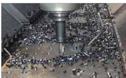
**Cutting condition**  $vc(\text{m/min})=70, fn(\text{mm/rev})=0.25, ap(\text{mm})=24$ , wet
